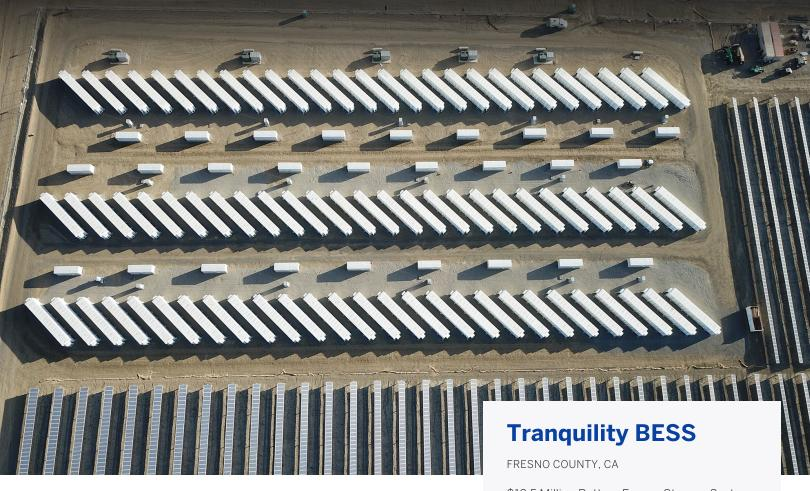
Rosendin was contracted by Recurrent Energy to design and build the \$12.5 million battery energy storage system (BESS) in Fresno County, California. This 72 MWac/288 MWh BESS project was added to the preexisting 200 MW Tranquillity Solar facility. Tranquillity BESS used Powin batteries to provide four hours of battery storage to the grid, enhancing resource capacity by conserving clean, solar energy to be used during peak demand.
